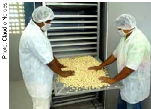
Figure 9. Cashew nut drying process in the minifactory.
