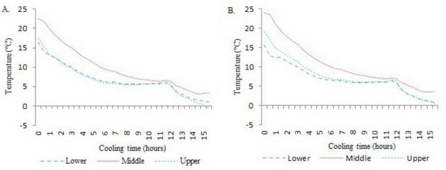
**Figure 2.** Air temperature as a function of cooling time at different heights within the same pallet: (A) pallet with polystyrene boxes and (B) pallet with cardboard boxes
