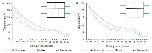
**Figure 3.** Air temperature as a function of cooling time at different positions in the pallet box layer (A) pallet with polystyrene boxes and (B) pallet with cardboard boxes
