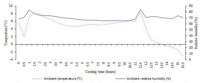
Figure 5. Ambient air temperature and relative air humidity during the period of operation of the forced air cooling room
