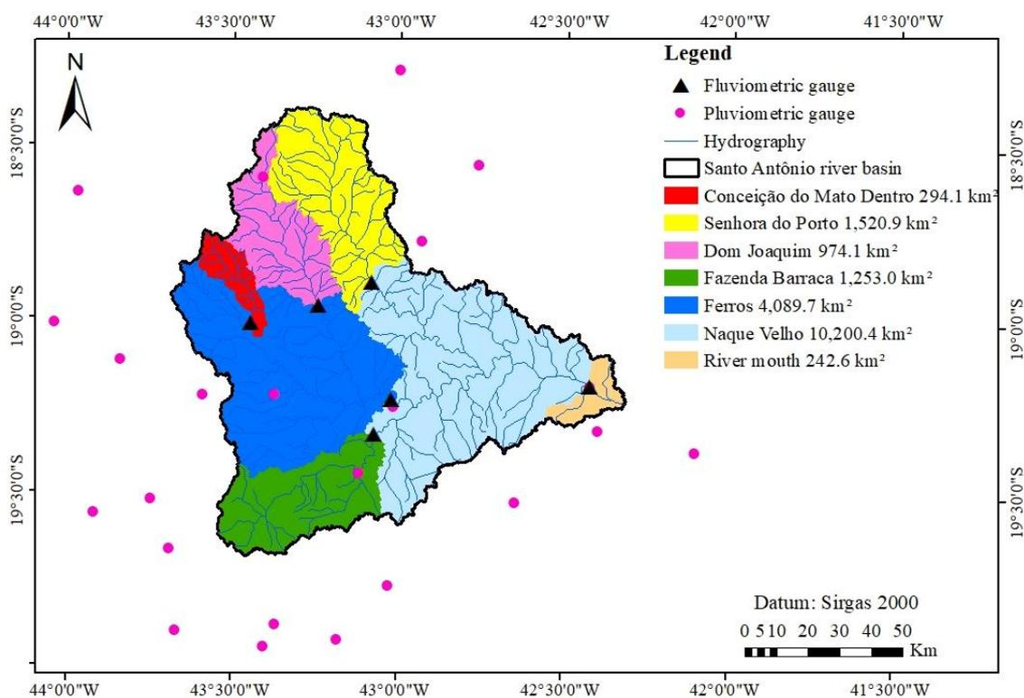
FIGURE 2. Fluvimetric gauges and their respective drainage areas, and rainfall gauges used.
