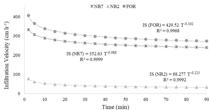
Fig. 4. Infiltration velocity ( $\text{cm h}^{-1}$ ) of soil water in a restoration area after bauxite mining under natural regeneration for two years (NR2), seven years (NR7), and a reference native forest (FOR), eastern Amazon, Brazil.
