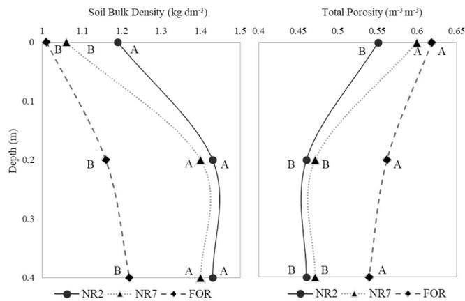
Fig. 3. Soil bulk density (Ds) and total porosity (Pt) in systems under natural regeneration for two years (NR2), seven years (NR7), and a reference native forest (FOR) in depths 0–0.1, 0.1–0.2, and 0.2–0.4 m, in a bauxite mining area in the eastern Amazon, Brazil.
