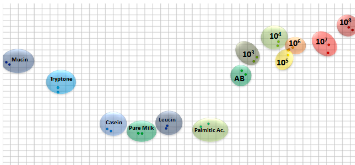
Fig. 5. IDMAP plot for the Electrical Impedance Spectra from interferents and milk solution in PBS and S. aureus antibody (AB).
