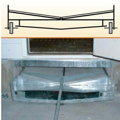
Figure 1. V-shaped scraper under one of the chambers.
