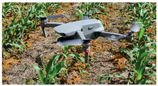
Figure 9. Drone with device to apply *Trichogramma* in corn.
