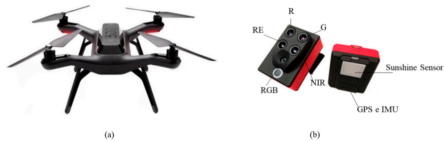
Figure 2. Equipment: (a) RPA used for the field survey; (b) camera, and sensors of imagery and irradiance.
