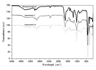
Figure 3. FTIR (ATR) spectra of bio-oils from raw biomass sorghum and experiments 7 and 15.
