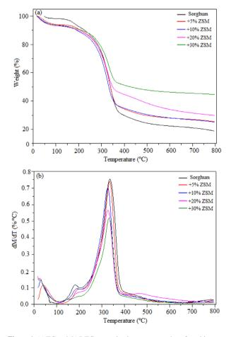
Figure 1. (a) TG and (b) DTG curves in nitrogen atmosphere from biomass sorghum, and sorghum + ZSM-5.
