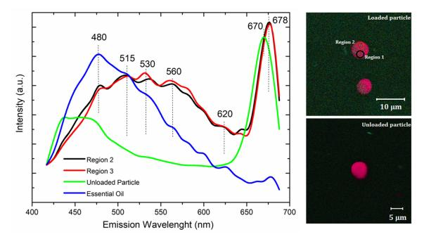
Figure 7. Fluorescence measurements of the loaded (regions 1 and 2) and unloaded particles.
