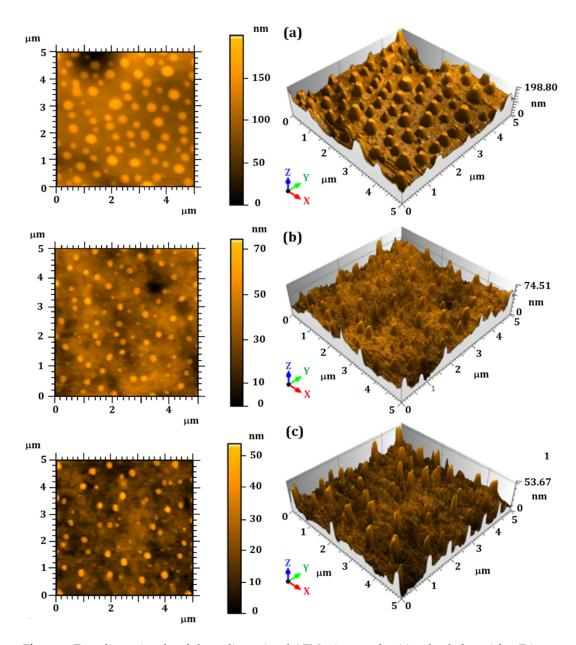
**Figure 1.** Two-dimensional and three-dimensional AFM micrographs: (a) unloaded particles ( $P_0$ ), (b) loaded particles using 500  $\mu$ g·mL<sup>-1</sup> of essential oil ( $P_{500}$ ), and (c) loaded particles using 1000  $\mu$ g·mL<sup>-1</sup> of essential oil ( $P_{1000}$ ).
