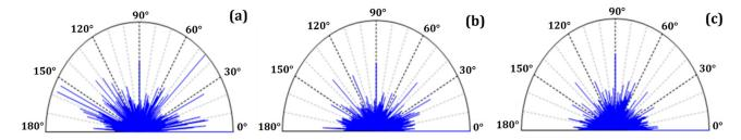
**Figure 4.** Surface texture directions for (a)  $P_0$ , (b)  $P_{500}$ , and (c)  $P_{1000}$ . All systems presented a similar microtexture, as the direct texture parameters did not show any statistically significant differences (p-value > 0.05).
