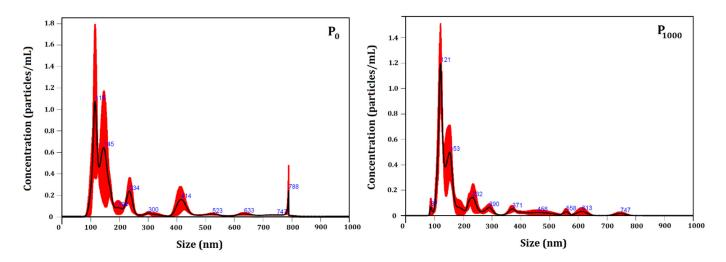
**Figure 5.** NTA particle size distribution analysis of  $P_0$  and  $P_{1000}$  systems. Representative histograms of the average size distribution (black line) from three measurements of a single sample. Red areas specify the standard deviation (SD) between measurements, and blue numbers indicate the maxima of individual peaks.
