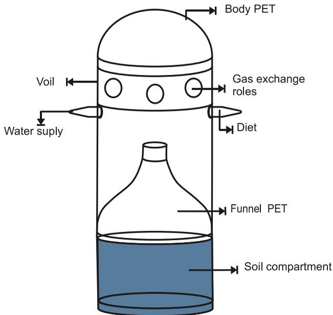
**Figure 1.** Cage developed for experiments evaluating the virulence of entomopathogens to fruit fly pupae. The lower compartment is built using PVC and can assume different lengths, receiving soil or substrate where larvae can be deposited. The aerial compartment, which was built using transparent PET, contains water and an artificial diet to receive emerging adults.
