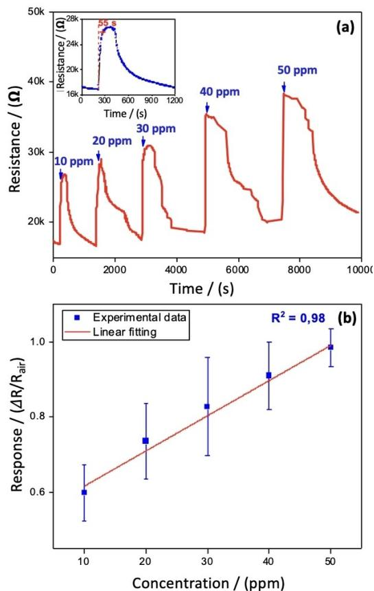
**Figure 8.** (a) Electrical response of TiO<sub>2</sub>/PANI nanocomposite towards different concentrations of ammonia. The inset shows the response time towards 10 ppm of NH<sub>3</sub>. (b) Linear dependence of response as a function of NH<sub>3</sub> concentration in the range 10–50 ppm. Gas response evaluated at 10 kHz and room temperature.
