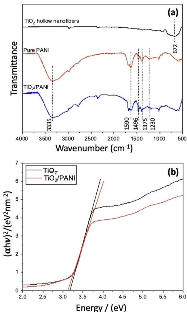
**Figure 3.** (a) FTIR spectra of:  $\text{TiO}_2$  hollow nanofibers, pure PANI and  $\text{TiO}_2$ /PANI composite. (b) Tauc's plot for band gap estimation of  $\text{TiO}_2$  and  $\text{TiO}_2$ /PANI composite.
