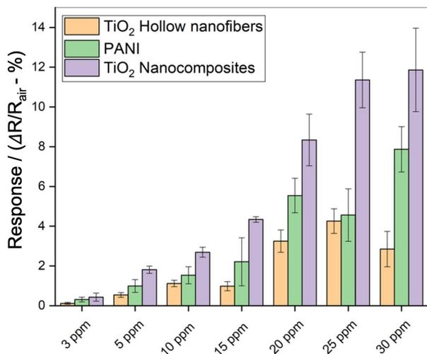
**Figure 6.** Electrical response of the three sensing platforms to different NH<sub>3</sub> concentrations.
