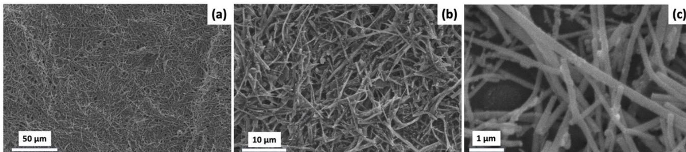
**Figure 4.** (a) SEM images of  $\text{TiO}_2$ /PANI composite deposited onto IDEs. (b) and (c) are magnified images.
