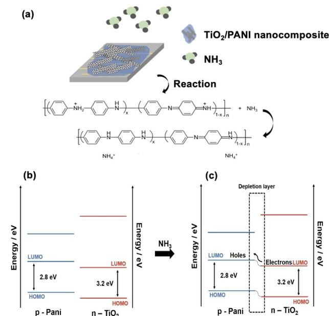
**Figure 9.** (a) Schematic representation of TiO<sub>2</sub>/PANI sensing and reaction mechanism. (b) Energy band diagram in air and (c) in the presence of NH<sub>3</sub>.<sup>[37]</sup>
