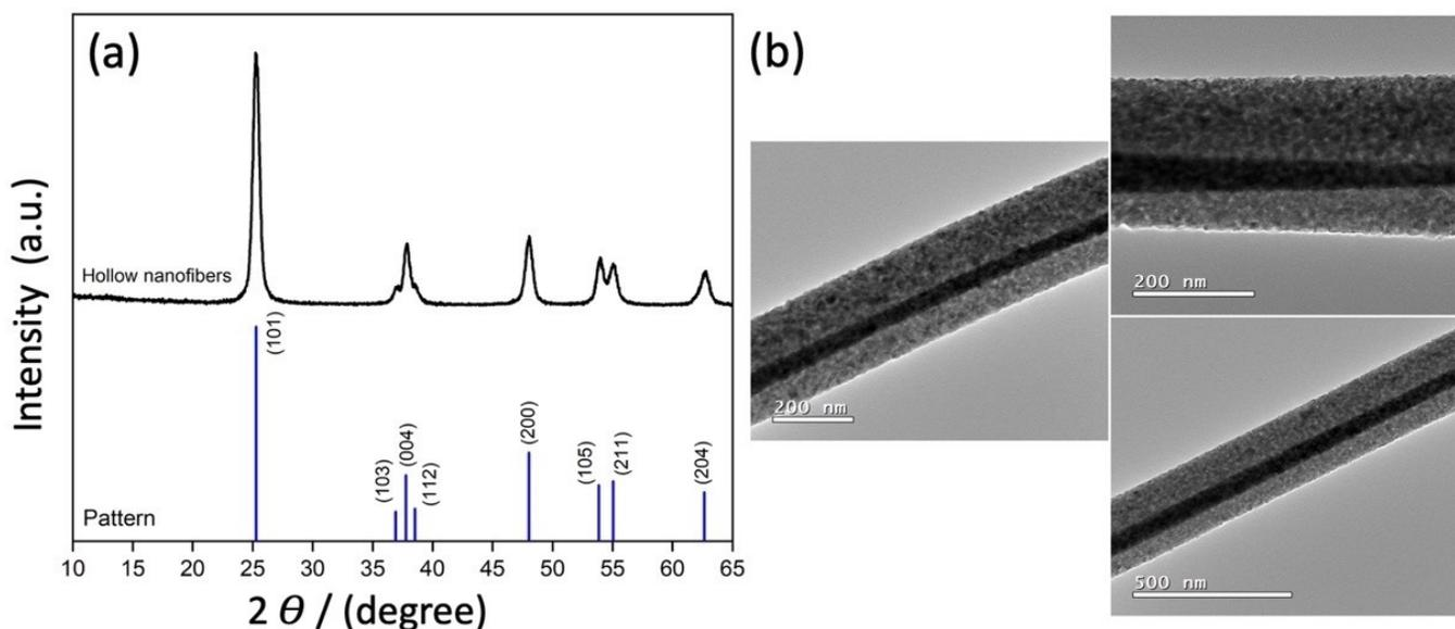
**Figure 2.** (a) XRD patterns of the hollow nanofibers, confirming crystalline  $\text{TiO}_2$  in the anatase phase. (b) Typical TEM images of a  $\text{TiO}_2$  hollow nanofiber.
