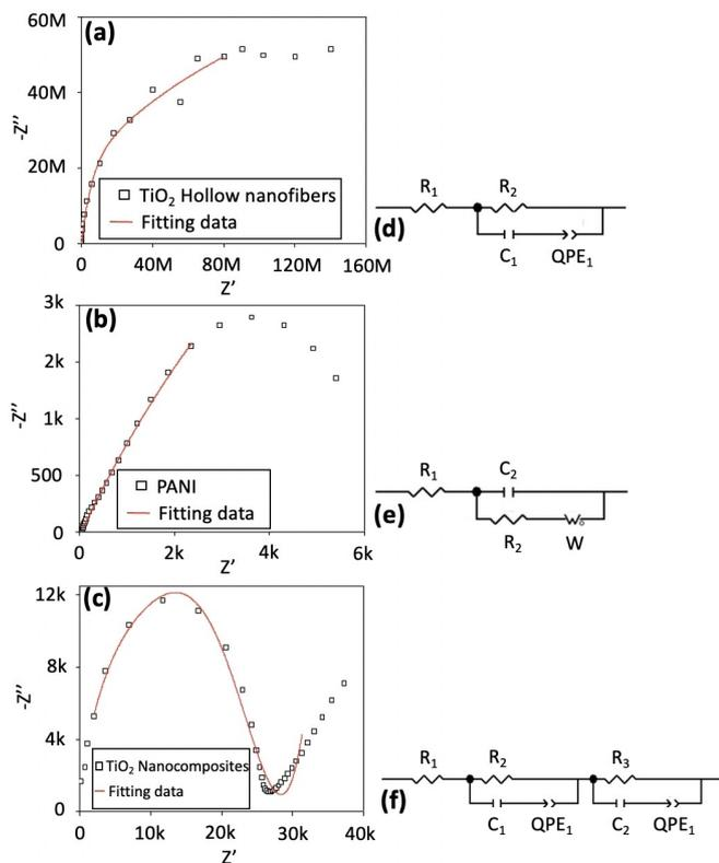
**Figure 5.** Nyquist diagram for (a) TiO<sub>2</sub> hollow nanofibers, (b) PANI, and (c) TiO<sub>2</sub>/PANI nanocomposites. Experimental data are shown by squares, while solid lines represent the fitting using the electrical circuits shown in (d–f).
