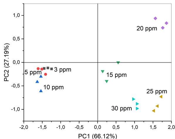
**Figure 7.** PCA graph for ammonia samples using average electrical resistance values, measured at 10 kHz, based on TiO<sub>2</sub>/PANI nanocomposite platforms.
