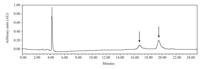
Figure 1. Chromatographic profile at 254 nm of *Lafoensia pacari* phenolics-containing extract. Column  $C_{18}$  (5  $\mu$ ; 250  $\times$  4.6 mm), mobile phase in a gradient system. Punicalagin  $\alpha$  and  $\beta$  anomers (arrows).
