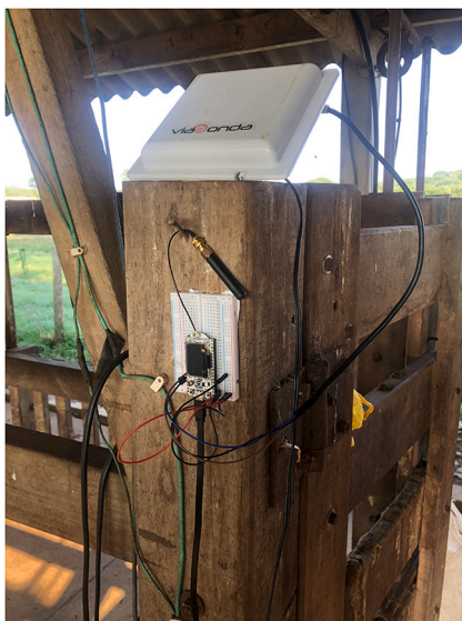
Fig. 6. Set of ESP32 Slave + Middle range presence sensor.
