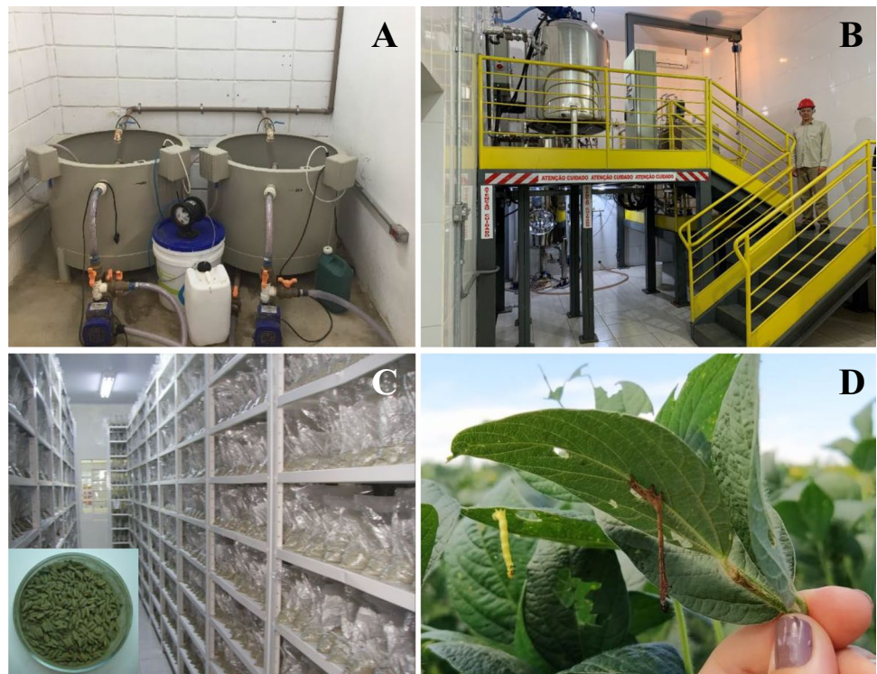
Fig. 1 On-farm liquid fermentation performed with limited (A) or extensive process control using a hermetic bioreactor (B) for fungal and bacterial microbes. On-farm production of fungi—solid-state fermentation in plastic bags filled with cooked rice grains (C). Baculovirus-infected caterpillars collected in a soybean field (D)
