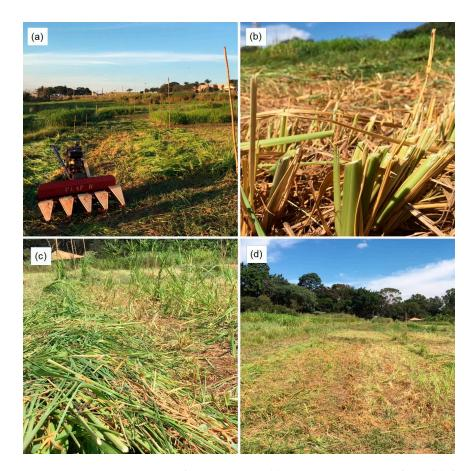
**Figure 10.** GRM's cutting type characterization: (**a**) Mini grain reaper machine; (**b**) the grass tussocks cut by this machine; (**c**) the piled-up grass biomass; (**d**) the grass plot after biomass removal.
