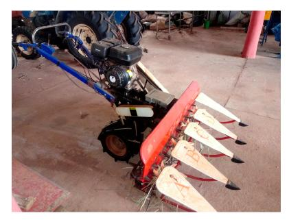
Figure 6. Mini grain reaper machine.
