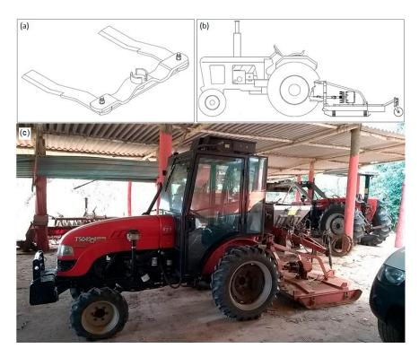
**Figure 5.** Tractor mounted rotary brushcutter: (**a**) rotating blades; (**b**) implement connected to the tractor's three-point system; (**c**) tractor and implement utilized.
