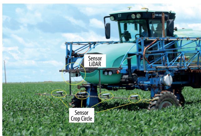
Figure 7. Use of LiDAR sensor in conjunction with Crop Circle® reflectance sensors, embedded in an implement for plant height detection.
