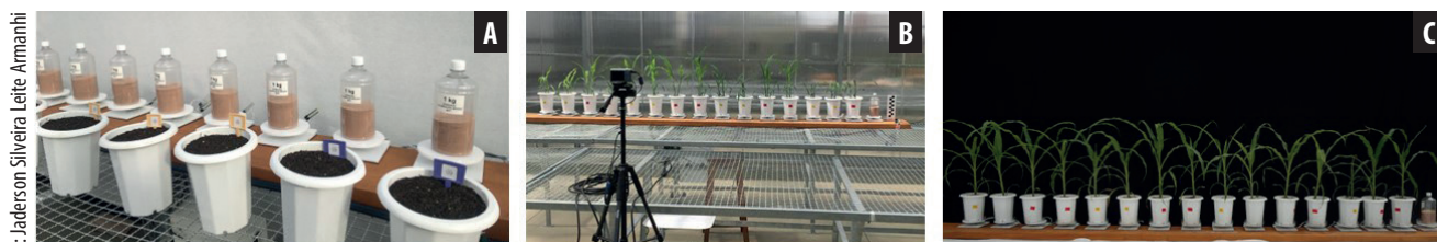
Photos: Jaderson Silveira Leite Armanhi Figure 5. Some aspects of the phenomics platform installed in the greenhouse. Scales and sensors installed for continuous monitoring of the weight of the pot-plant system and soil/substrate moisture (A); camera installed to continuously record plant growth (B); corn plants monitored continuously in the experiments carried out (C).
