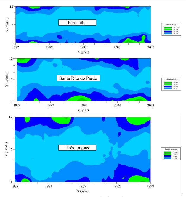
FIGURE 5. Temporal distribution of rainfall erosivity (R; MJ mm h<sup>-1</sup> ha<sup>-1</sup> month<sup>-1</sup>) over months and years in the municipalities of the Bolsão region of Mato Grosso do Sul (Brazil), except for Selvíria.
