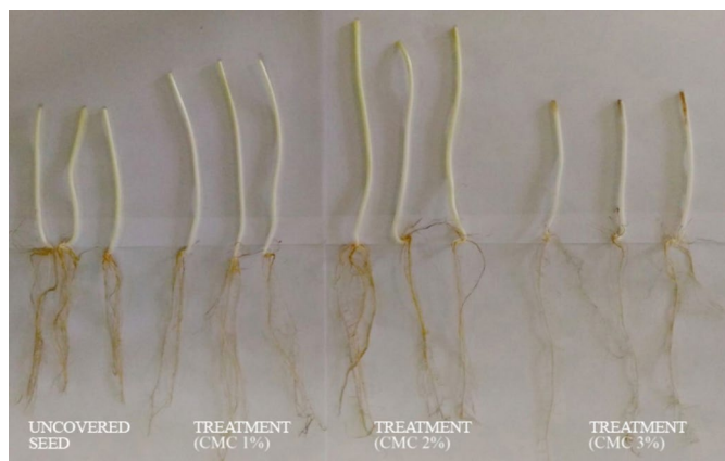
Figure 6: Seedling length from seeds coated with different concentrations of carboxymethyl cellulose.
