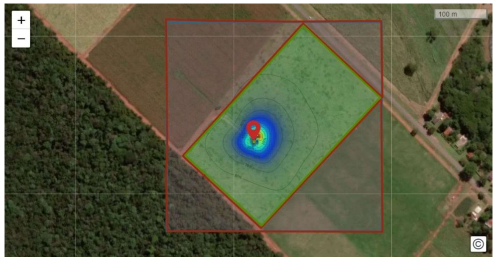
Fig. 5 Study site geographic location: Santo Antônio de Goiás, in the state of Goiás, Brazil. The true-color Google Earth image from 2021, in EPSG: 4326—WGS84, was used as the base map. Additionally, the footprint contribution area of the eddy covariance (EC) method was overlaid to analyze the influence of the surrounding land cover on the evapotranspiration measurements
