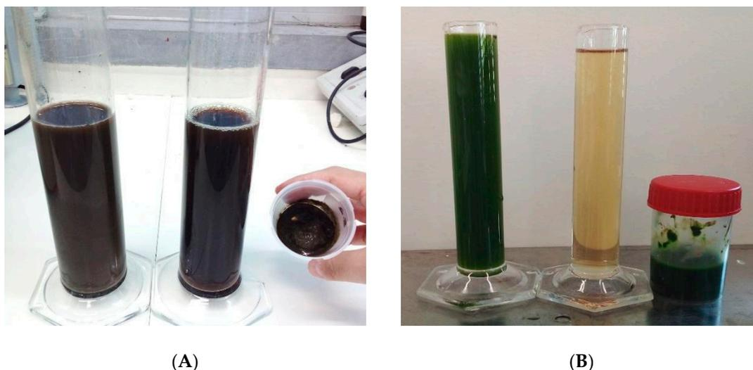
**Figure 6.** Samples were centrifuged and then freeze-dried. **(A)** Anaerobic digestate biomass, sample treated by co-digestion. **(B)** Microalgae biomass, sample treated by photobioreactors. The supernatant was characterized to evaluate the bioremediation performance of the microalgae.
