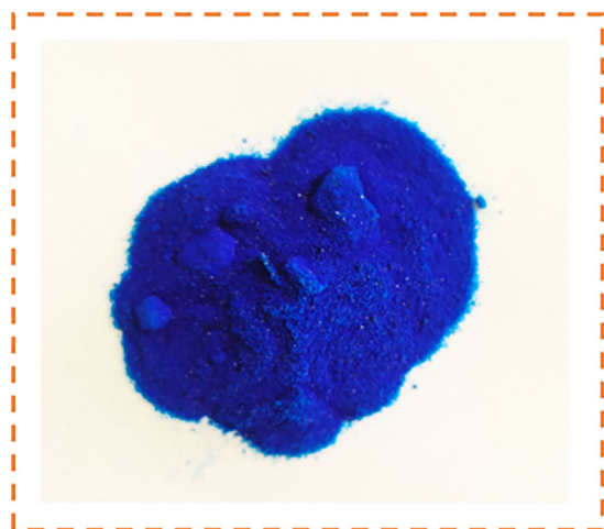
Figure 10. Photography of Cu-based MOF HKUST-1.
