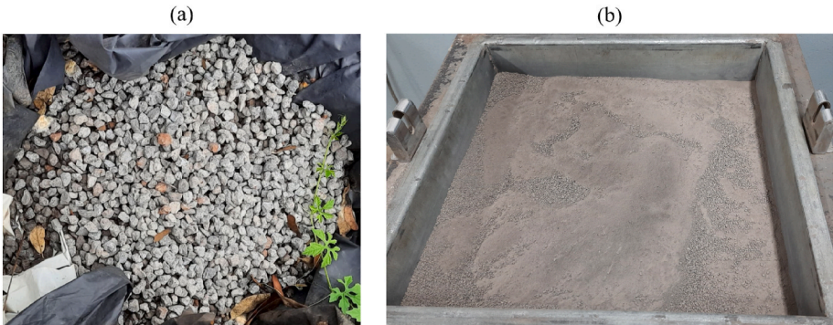
Fig. 4. BOFS: (a) before grinding; (b) after grinding and sieving.
