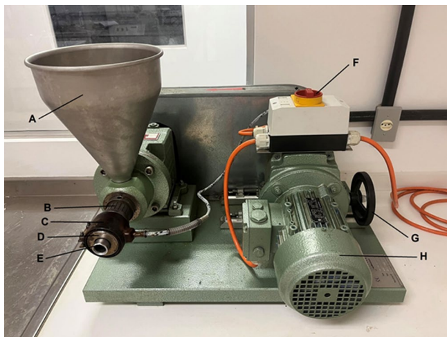
FIGURE 1 | Expeller press used in the experiments, (A) feed hopper, (B) perforated cylinder (oil outlet), (C) strip heater, (D) screw head, (E) outlet nozzle of press cake, (F) start button, (G) gearbox, (H) motor.
