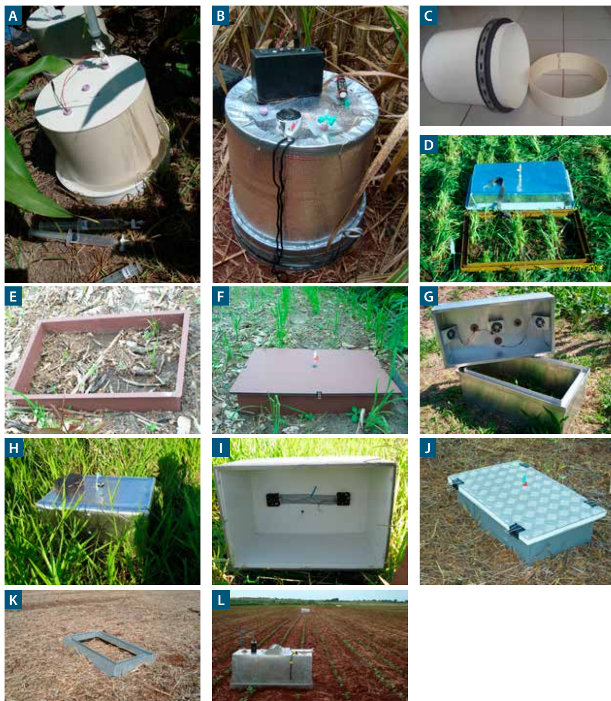
Figure 4.4. Types of chambers and materials available for fabrication: (A) cylindrical shape with galvanized steel base and PVC top; (B) cylindrical shape with galvanized steel base and polyurethane top covered with thermal insulation; (C, D) cylindrical shape with PVC base and top; (E) rectangular shape with galvanized steel base and polyethylene top; (F) square shape with galvanized steel base and top; (G) rectangular shape with aluminum base and top; (H) rectangular shape with galvanized steel base and polypropylene top covered with thermal insulation; (I) rectangular shape with galvanized steel base and top; and (J) rectangular shape with galvanized steel base and polyethylene top.
