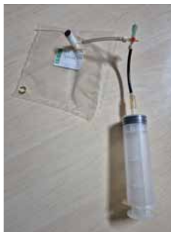
Figure 4.8. Transferring air from the chamber to the Tedlar bag using a 200 mL syringe. Note that an initial aspiration of 10 mL is carried out for flushing, followed by aspiration and transfer of 200 mL of air from the chamber into the bag. The bags are then taken to the laboratory and individually connected to the laser analyzer, where nitrous oxide ( \text{N}_2\text{O} ) and methane ( \text{CH}_4 ) concentrations are analyzed in approximately 1.5 minutes
