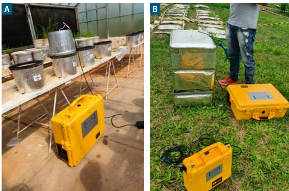
Figure 4.6. Off-axis integrated cavity output spectroscopy (OA-ICOS) analyzer for monitoring nitrous oxide ( \text{N}_2\text{O} ) and methane ( \text{CH}_4 ) flows in soil planted with soybeans, in a greenhouse (A) and in the field (B), both at Embrapa Agrobiologia.
