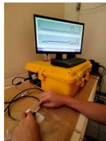
Figure 4.8. Transferring air from the chamber to the Tedlar bag using a 200 mL syringe. Note that an initial aspiration of 10 mL is carried out for flushing, followed by aspiration and transfer of 200 mL of air from the chamber into the bag. The bags are then taken to the laboratory and individually connected to the laser analyzer, where nitrous oxide ( \text{N}_2\text{O} ) and methane ( \text{CH}_4 ) concentrations are analyzed in approximately 1.5 minutes
