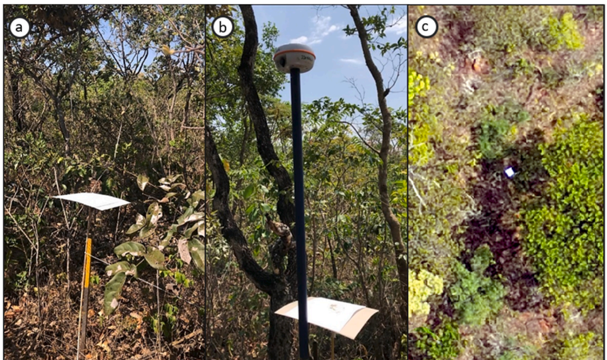
Fig. 3. a) Ground control point (GCP) at the vertex of the permanent plot, made with cardboard and a white sheet. The white sheet aimed to ensure good reflectance for identification in the image captured by the DJI Phantom4 Pro; b) Geodetic DGPS collecting X, Y coordinates and Z elevation of the permanent plot vertices; c) visualization of the target in the orthomosaic.
