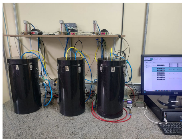
EXHIBIT 4 | Experimental setup of the laboratory bioreactor system. [Color figures can be viewed at wileyonlinelibrary.com .]
