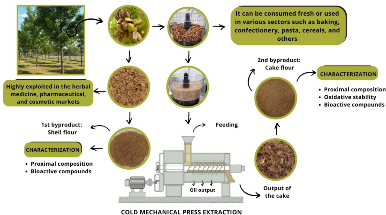
Figure 1. Diagram illustrating the cold mechanical press extraction process of pecan oil and the generation of byproducts
