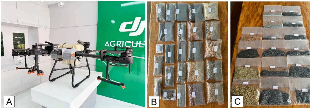
Figure 2. (A) DJI Agras T30 drone equipped with a solid spreader tank for seeding, (B) seeds of forest species, and (C) seeds for pastures and soil cover.
