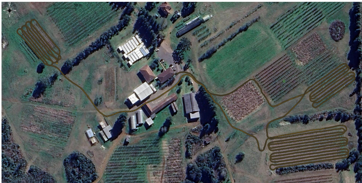
Figure 2. The positions registered by the GNSS RTK module in the mission performed on March 11, 2025, at Embrapa's Temperate Climate Fruit Growing Experimental Station, Vacaria, RS.
