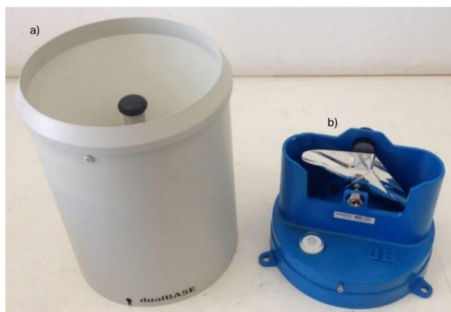
Fig. 3 Funnel (a) and buckets (b) of the DualBase PluviDB rain gauge instrument installed on the tower [7]
