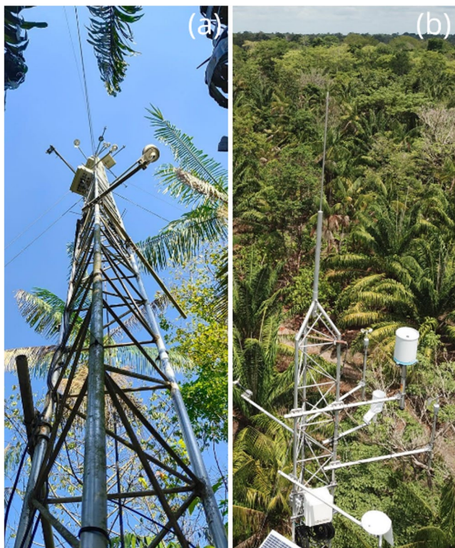
Fig. 2 Micrometeorological observation tower in the municipality of Tomé-Açu, Pará (a); Location of the tipping bucket rain gauge. (b) Source: Giselle Nerino (a); Leonardo Ramos (b)
