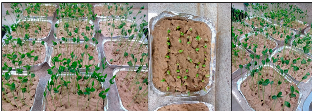
Figure 4. Soybean seeds that had emerged (seedlings) were subjected to germination testing after passing through the pneumatic seed metering system at different sowing speeds and longitudinal inclination angles. Prepared by the authors.
