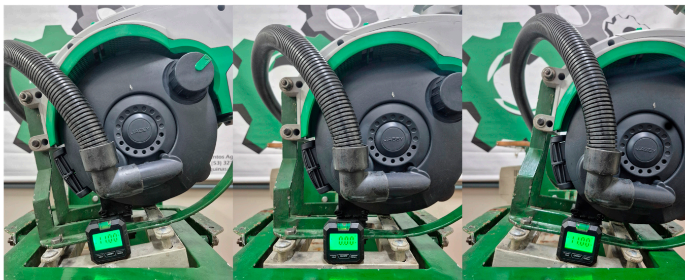
Figure 1. Pneumatic seeder at inclinations of 11°, 0° and −11°, respectively.
