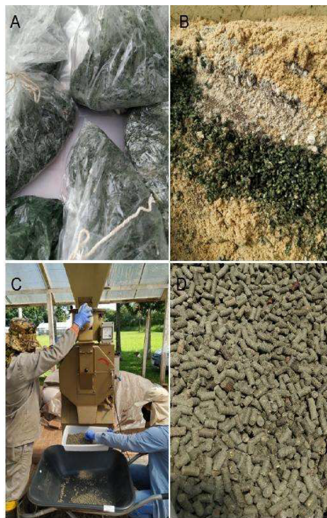
Figure 1. Bioactive matrix of T. harzianum (A), mixture for pelletization (B), pelletizing device (C), and organomineral pellets containing T. harzianum (D).
