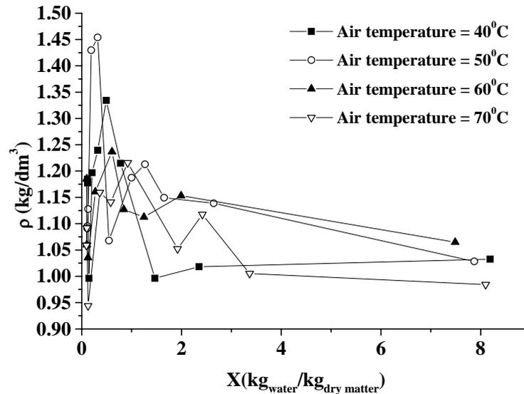
Fig. 4. Samples bulk density as a function of their moisture content at several air temperatures.
