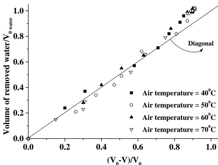
Fig. 3. Volume of removed water as a function of samples volume.
