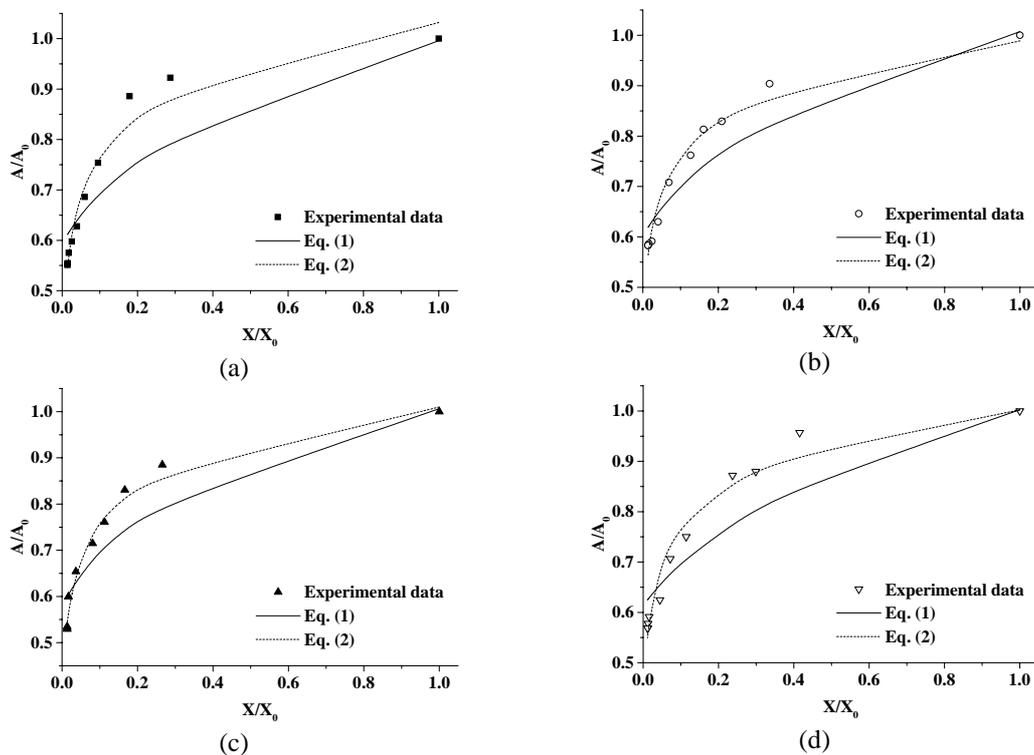
Fig. 6. Modelling of shrinkage kinetics, during drying process of papaya slices, using Eqs. (1) and (2) at (a) 40<sup>o</sup>C, (b) 50<sup>o</sup>C, (c) 60<sup>o</sup>C and (d) 70<sup>o</sup>C.
