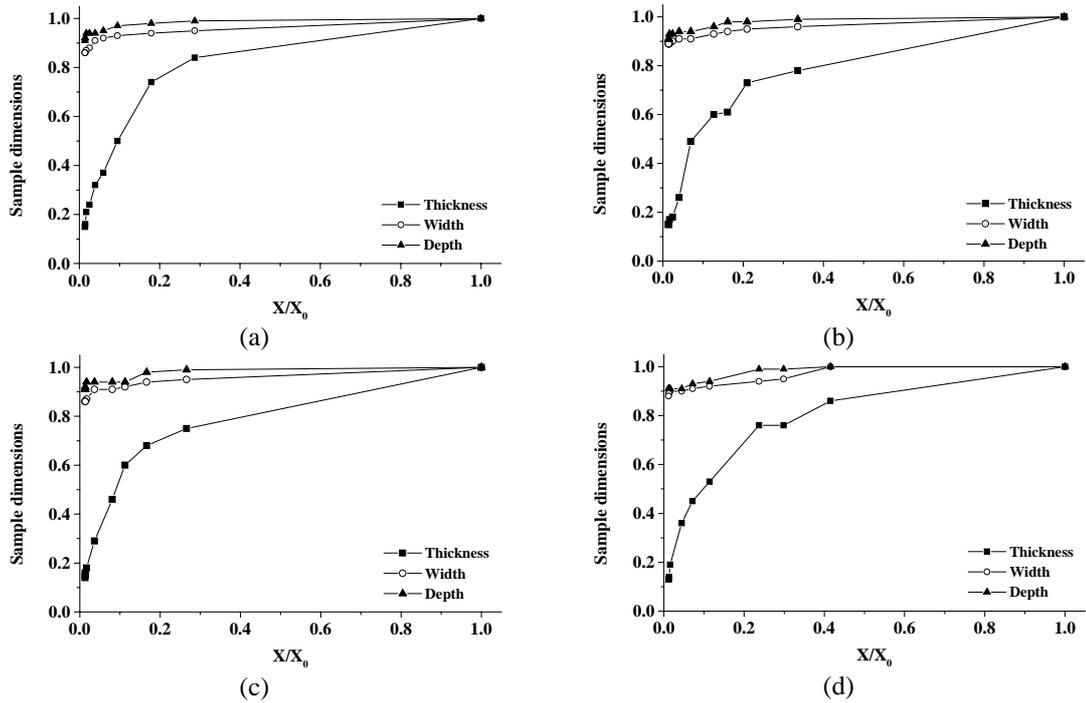
Fig. 5. Variation in samples dimension as a function of their moisture content at (a) 40<sup>o</sup>C, (b) 50<sup>o</sup>C, (c) 60<sup>o</sup>C and (d) 70<sup>o</sup>C.
