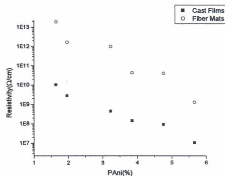
Figure.3- Volumetric resistivity of PANi-TSA/PLA electrospun fiber mats and the correspondin casting films.
