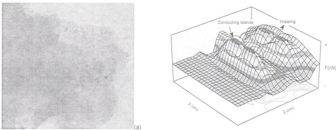
Figure 1. (a) TEM micrograph of POEA highly doped (pH=3.0), magnification (x100.000) and (b) Adhesion map obtained by AFS on POEA films in solution (pH=3.0). The charge nanocarriers hopping occur between two nearer conducting islands.
