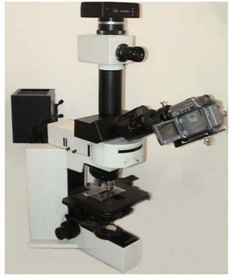
Figure 1. Coupling of digital camera to the microscope.
