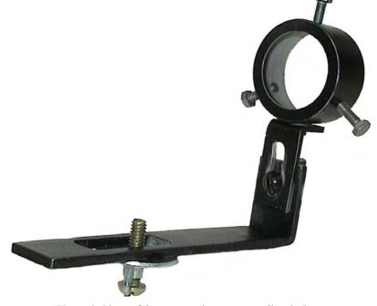
Figure 3. Photo of the camera microscope coupling device.
