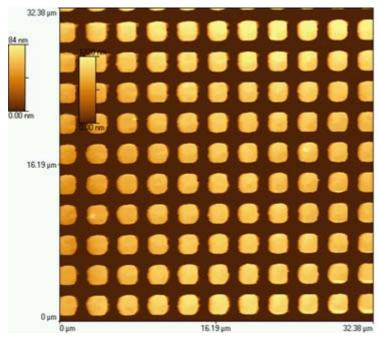
Figure 7. AFM image of the calibration grid with 8.000 times magnification.
