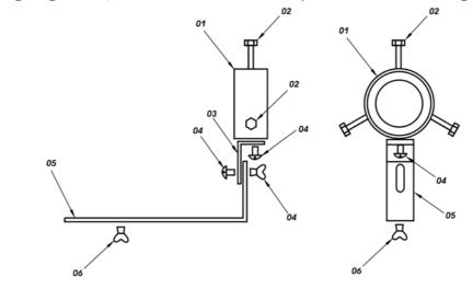
Figure 2. Diagram of the camera microscope coupling device.
