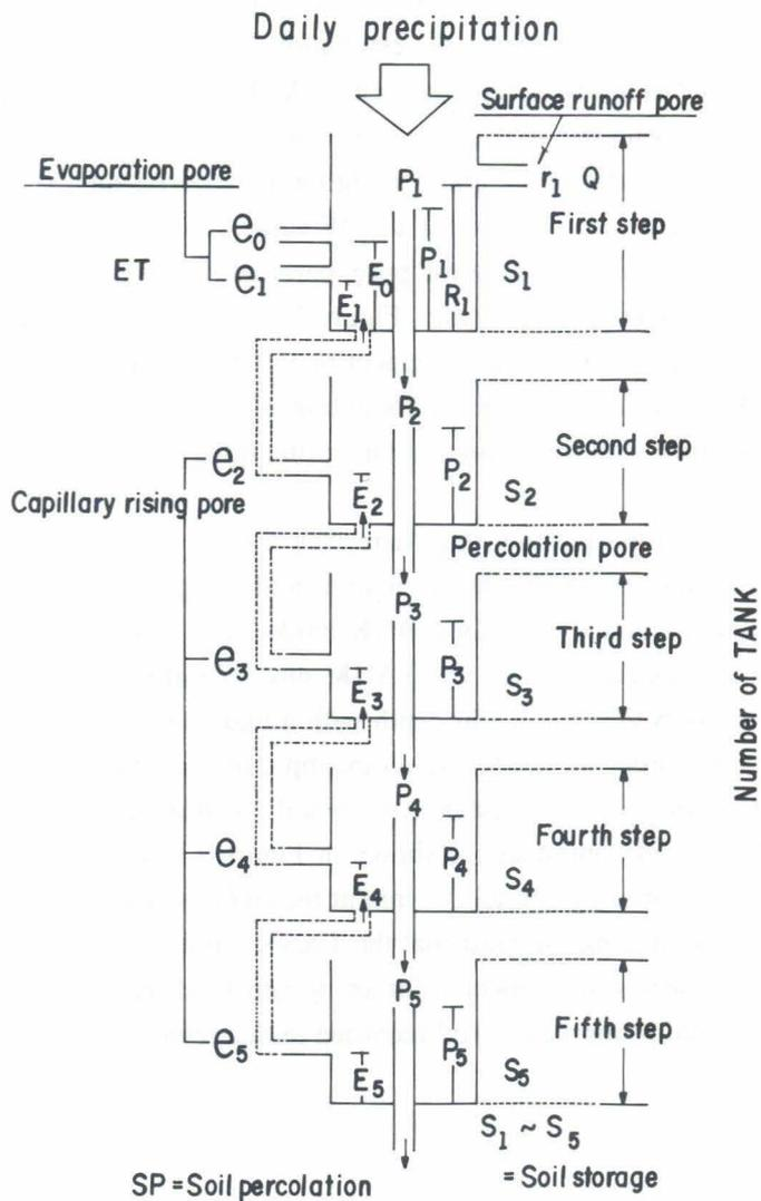
FIG. 8 - Schematic illustration of the "TANK" model.
