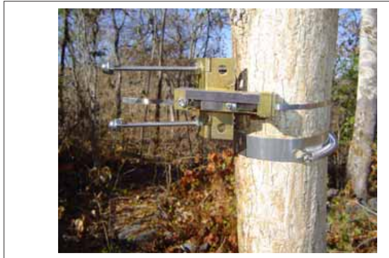
Fig. 1. Imported industrial (above) and national home made (bellow) dendrometer bands used to measure growth in trunks of Acacia tenuifolia in a seasonally dry forest in Central Brazil.
