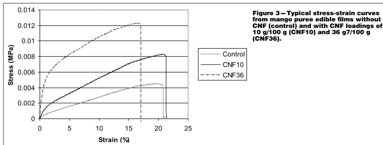
**Figure 3 – Typical stress-strain curves from mango puree edible films without CNF (control) and with CNF loadings of 10 g/100 g (CNF10) and 36 g/100 g (CNF36).**
