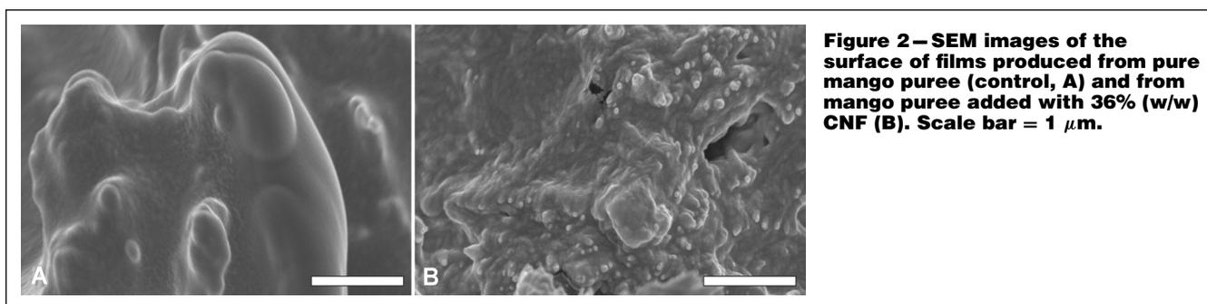
**Figure 2 – SEM images of the surface of films produced from pure mango puree (control, A) and from mango puree added with 36% (w/w) CNF (B). Scale bar = 1  $\mu$ m.**
