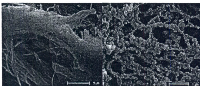
Figure 1: FEG-SEM image of polyaniline film obtained with the pressurized fluid method.
