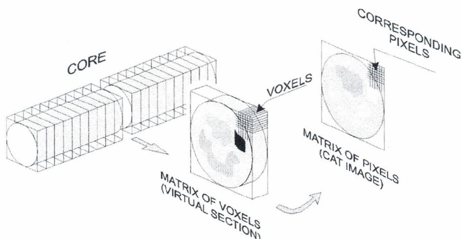
Figure 2. Schematic representation of image reconstruction (Duliu, 1999).
