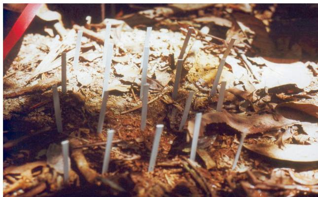
Fig. 2: Description of the bait-lamina tests system (VON TÖRNE 1990): Left: Individual test sticks showing the holes which contains the feeding material; right: bait-lamina sticks in the litter of a primary forest soil
