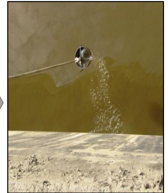
C) & D) Filling and retrieving the container with river water.
