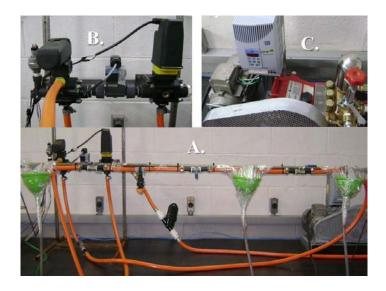
**Fig. 3**. Hydraulic circuit and components. A. general view; B. from left to right: pressure sensor, on/off valve, flow sensor and proportional flow valve; C. electric motor, frequency inverter and hydraulic piston pump.
