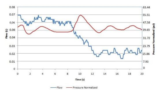
**Fig. 10**. Flow and pressure in a 3 nozzles system when the flow in 2 nozzles was obstructed.
