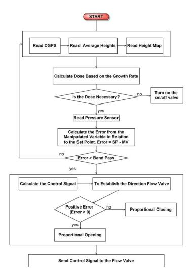
Fig. 4. Flow Chart of Pressure valve Controller Software
