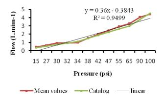
Fig. 5. Varitarget calibration curve
