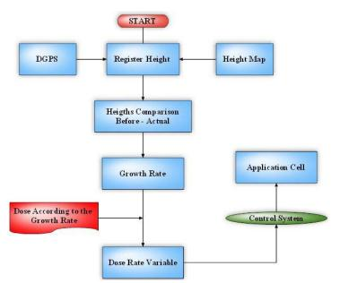
Fig. 1. Flow chart of the mepiquat control application system.
