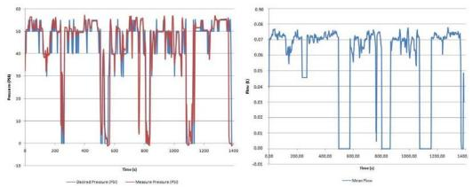
**Fig. 9.** Desired pressure and measure pressure during a simulation period (a) and the mean flow over the same period (b) at sprayer forward speed of  $2.5 \text{ m.s}^{-1}$ .
