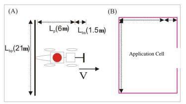
Fig. 2. Control cell for mepiquat application.
