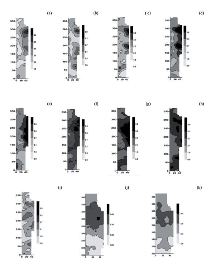
**Figure 5.** Maps for resistance penetration of soil 0.0-0.4 m depth: (a) Strokes of number; (b) Resistance kPa 0.0-0.05 m; (c) Resistance kPa 0.05-0.10 m; (d) Resistance kPa 0.10-0.15 m; (e) Resistance kPa 0.15-0.20 m; (f) Resistance kPa 0.20-0.25 m; (g) Resistance kPa 0.25-0.30 m; (h) Resistance kPa 0.30-0.35 m; (i) Resistance kPa 0.35-0.40 m. Maps for soil density (kg m<sup>-3</sup>): (j) 0.0-0.20 m of the depth; (k) 0.20-0.40 m of the depth.
