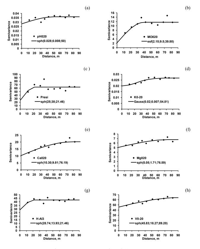
**Figure 3.** Semivariograms for soil chemical attributes 0.0 a 0.20 m of the depth: (a) pH; (b) M.O.; (c) P; (d) K<sup>+</sup>; (e) Ca<sup>2+</sup>; (f) Mg<sup>2+</sup>; (g) H+Al<sup>3+</sup>; (h) V%.
