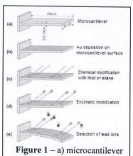
Figure 1 – a) microcantilever characteristics and (b, c, d, e) construction steps of device.
