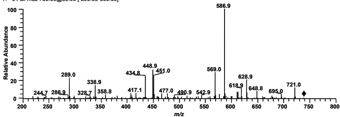
**Figure 5.** Product ion spectrum of the precursor ion  $[M - H]^-$  at  $m/z$  739 of a dimeric B-type C-glycosylated procyanidin identified in the infusion from the barks of *H. speciosa* in collision energy of 30%.
