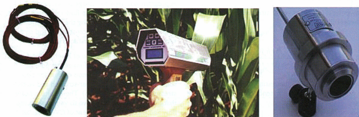
Figure 13. Infrared thermometer transducer models commonly used in the canopy-air temperature difference measurements (from left to right: Apogee IRTS-P5, Telatemp AG510b, and Everest Intersciences 4000.3ZL).
