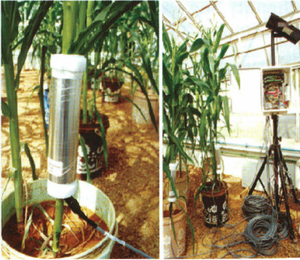
Figure 14. Energy balance probe (left) and automatic sap flow measurement system, installed on stem sections of eight maize inbred line plants to measure the transpiration rate and water stress levels at the Sete Lagoas site (Source: Gomide et al, 2005).
