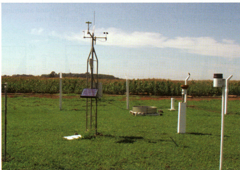
Figure 6. Automatic weather station installed in the Sete Lagoas specific site for local microclimate characterisation, ET_0 determination, and irrigation water management.
